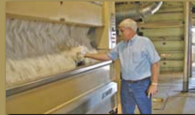
Dirt, seeds, hulls and other particles are removed from the cotton as it runs through the cotton gin, also called ginning.
